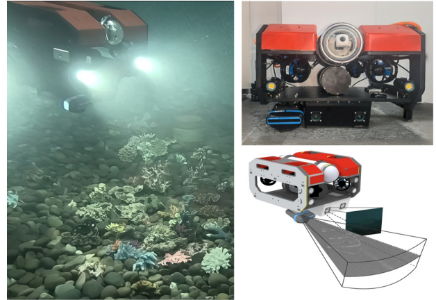
Fig. 1: The SonarSweep System. (Left) The experimental AUV in a challenging underwater environment. (Top Right) The integrated camera and sonar sensor suite. (Bottom Right) Conceptual diagram of the fusion approach.
