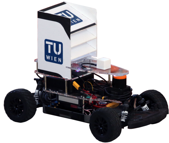
Fig. 4. F1Tenth experimental platform with Asus NUC and Hokuyo LiDAR.
