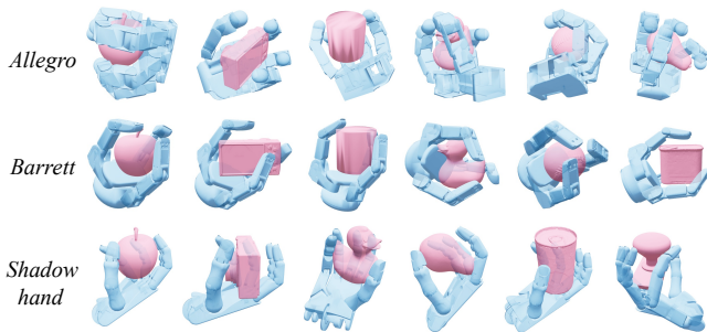
Fig. 3: Diverse and accurate unconditioned grasp synthesis of \mathcal{T}(\mathcal{R}, \mathcal{O}) across multiple dexterous hand embodiments.
