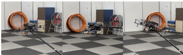
Fig. 9. The quadrotor is disturbed by a series of external forces via a push-rod.
