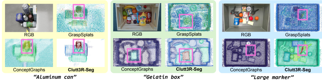
Fig. 8: Qualitative result of language-grounded semantic segmentation. Left: synthetic dataset. Middle, Right: GraspClutter6D dataset. Red color indicates high similarity, and target object is highlighted in the pink box.
