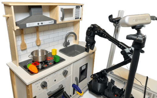
Fig. 3: WidowX Robot Arm Setup. We evaluate the scalability of HAND on 10 manipulation tasks on a WidowX robot arm in a kitchen setup [43].
