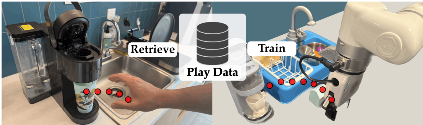
Fig. 1: HAND learns a policy from as little as 1 human hand demonstration and 4 minutes of real-world time by retrieving from robot play data.
