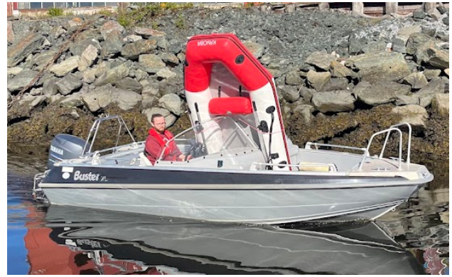
Fig. 5: Obstacle vessel used in the closed loop experiments. The vessel was augmented to compensate for limited 16-ray LiDAR resolution.
