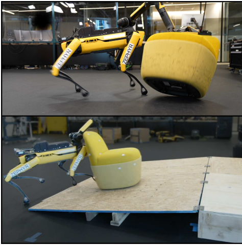
Fig. 5: A Spot robot uses its whole arm to upright a fallen chair (top). Spot pushes a chair up a ramp while making contact with multiple parts of its body (bottom). A low-level policy controls the locomotion, while judo samples high-level base velocity and arm commands for manipulation.
