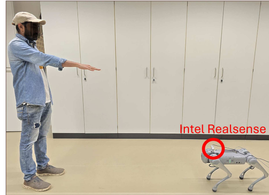
Fig. 1. Illustration of human–robot interaction scenario: a participant executes predefined actions while engaging with the Unitree Go1 robot, forming part of the dataset collection for action recognition and HRI analysis.
