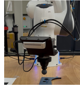
Fig. 3: Custom end-effector mount for the Franka Emika Panda integrating a force-torque sensor and provisions for RGB-Depth camera. A spherical tool tip enables smooth circular motion within holes. (Scenario 2, Sec. V-D)
