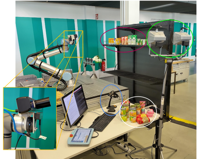
Fig. 1. General physical setup: Two calibrated RGB-D cameras (yellow) mounted on the robot end-effector view at the shelf; the camera pose in the image captures the iterative (image, SKU) pairs. A handheld barcode scanner (blue) records SKUs; a staging area holds upcoming products (white); a controllable studio light varies illumination (green); and already placed objects in the shelf are indicated in purple.
