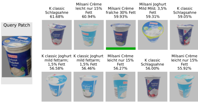
Fig. 4. Top- k results (right) sorted by similarity score from top left to bottom right for a given scene image crop of a segmented object proposal (left). Besides views of the correct object (green underline) we also get views of similar-looking objects (note that the different dark blue object renderings do not belong to the same object - they are near-duplicates).
