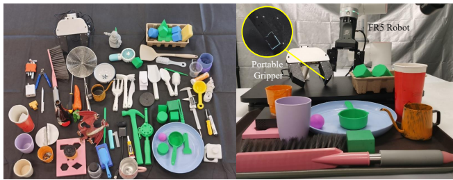
Fig. 4: Experimental setup for our system. For the right part, the top half shows the robot and portable gripper, which uses the same tactile device. The bottom half shows our experimental objects. We display the camera setting in Fig. 2. For the left part, the image shows a subset of the objects we used to collect our large-scale tactile image dataset.
