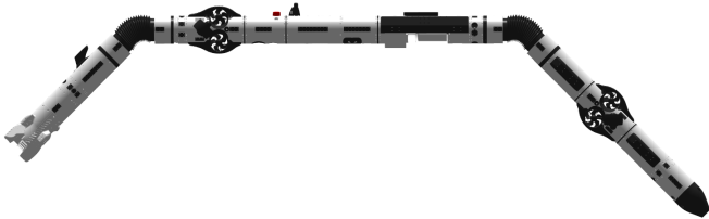
Fig. 1. Render of the Eelume 500 AIAUV (Eelume-M). Its “head” is to the left and its “tail” is to the right.
