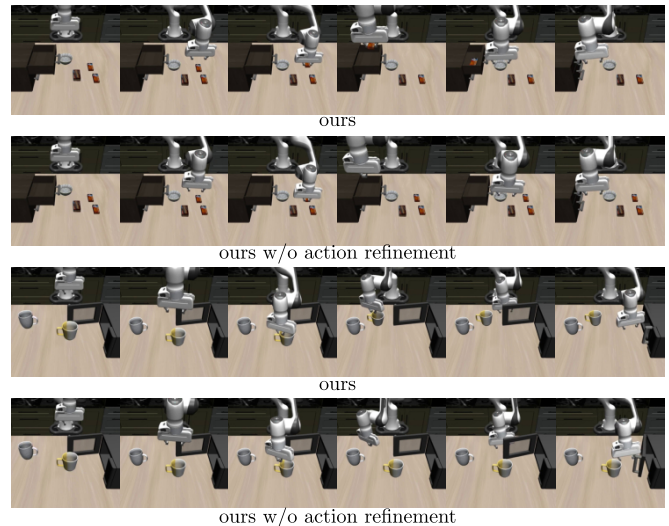
Fig. 5. Rollout comparison between our model and the variant without action refinement. The model without action refinement produces coarse actions that merely reflect the general trend of the task but remain imprecise; action refinement enhances precision and enables successful completion.
