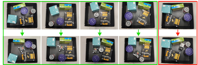
Fig. 4. Overhead views of 5 of the 40 packing scenes used during hardware experiments. Top row shows the state of the scene before packing and the bottom row shows the state of the scene after the object (tomato passata) was packed inside the container. Four of these trials were successful (green outline) and one was unsuccessful (red outline). The unsuccessful case was an object detached failure, hence the object is in a different orientation.
