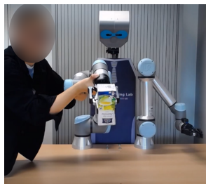
Fig. 2: Kinesthetic teaching of the throwing kernel. A human demonstrator physically guides the robot arm through a throwing motion. This provides a safe initial kernel that bootstraps RL training and avoids unsafe random exploration.
