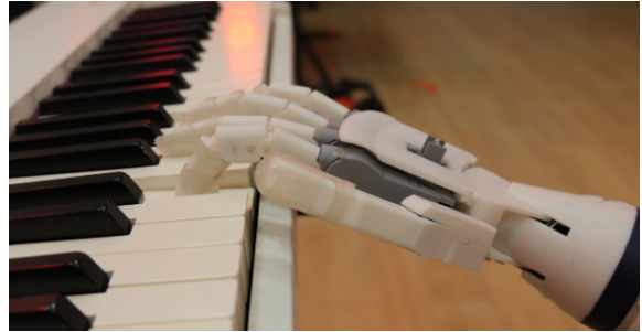
Fig. 1: The developed robotic prosthetic hand. The system features independent finger control, adjustable finger spacing, and a 2D wrist optimized for keyboard typing and piano playing applications. All components are 3D-printed with affordable electronics and actuators.
