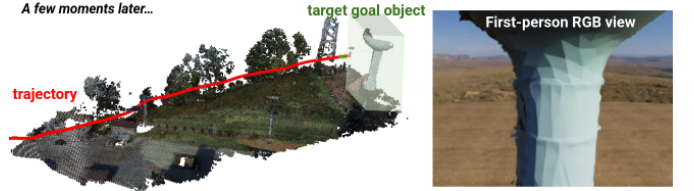
Fig. 3: (a) When no information exists within depth range, the robot activates semantic ray navigation for long-range coarse search, using ray features where the tower was briefly captured in the RGB view. (b) As it follows the rays and approaches the target, voxels naturally form and the search transitions to precise voxel-based navigation.
