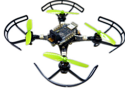
Fig. 3. The Crazyflie 2.1 Brushless nano-drone used in our experiments.
