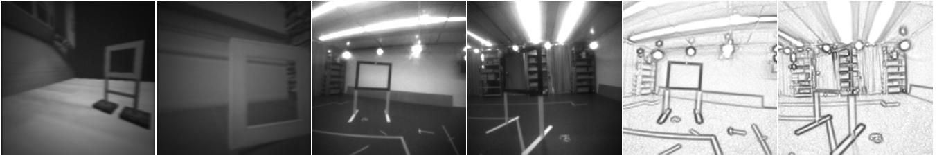
Fig. 4. Examples of (left) simulated images from \mathcal{D}_{\text{sim}}^{\text{train}} , (middle) real-world robot images in \mathcal{D}_{\text{real}}^{\text{train}} , and (right) after applying the pencil filter [6].
