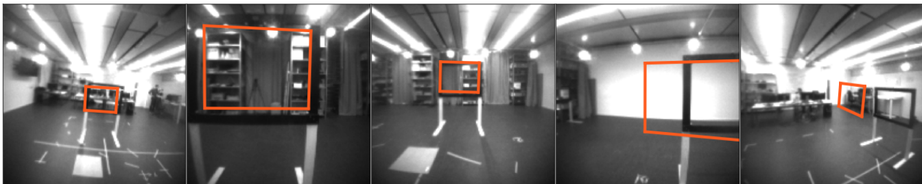
Fig. 6. Input frames overlaid with gate skeleton (in orange) using the pose predicted by our approach. The model correctly locates the gate (1-3), while failures occur when a large portion of the gate is occluded and for shallow angles (4-5).
