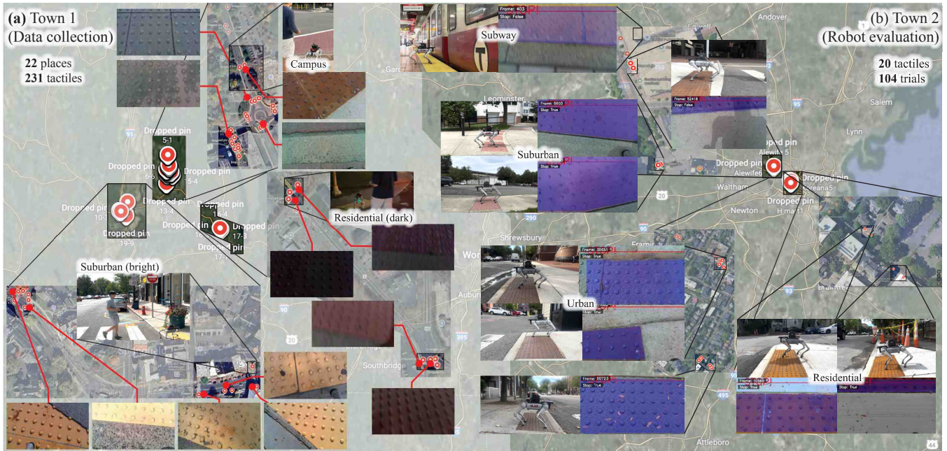
Fig. 3. Real robot data collection and hardware experiment. (a) We collected data with a quadruped robot across multiple sites in suburban, campus, and rural environments featuring various truncated domes. Data were gathered at different times of day under diverse truncated dome appearances. (b) We evaluated the robot’s reliable stopping at truncated domes in unseen areas. We present the hardware experiment setup and segmentation inference results.
