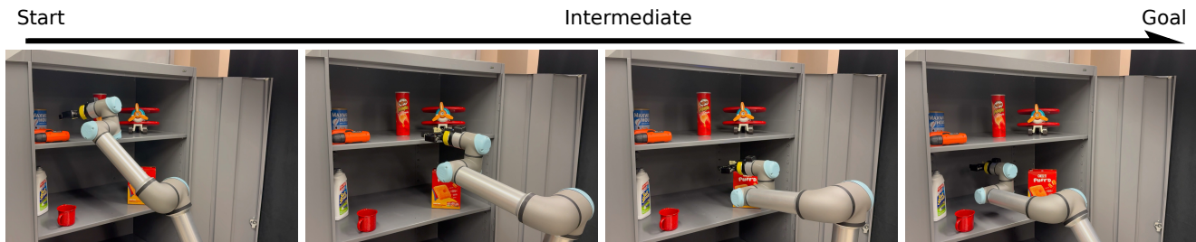
Fig. 5: Demonstration of a planned path where the robot arm navigates through a complex cabinet environment.
