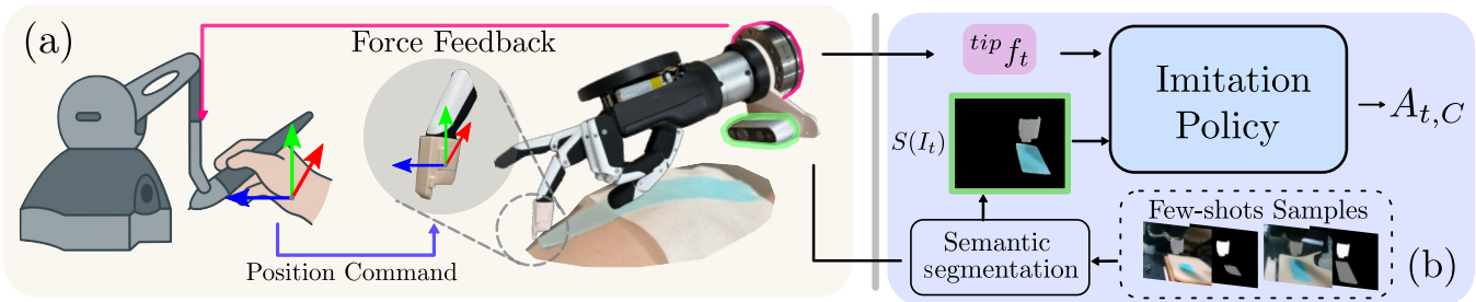
Fig. 2: The tape initial detachment framework includes (a) demonstration data collection via human teleoperation and (b) imitation learning for training and inference. An operator uses a haptic device to control the robot tip, receiving force feedback from a sensor between the hand and arm, while in-hand cameras capture images. The network is trained on segmented image and force data to predict future tip movements or forces, with semantic segmentation initialized from a small set of labeled samples.
