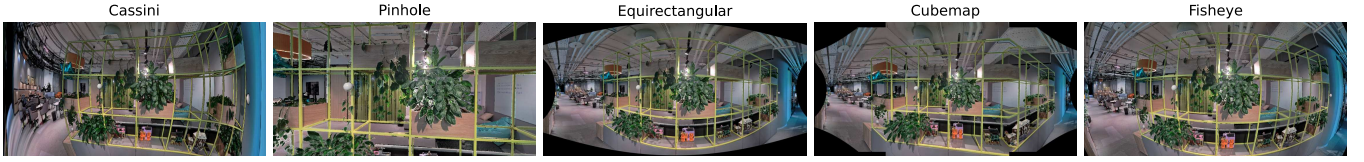
Fig. 1. Benchmark scene presented in the considered projections: Cassini, Pinhole, Equirectangular, Cubemap, Fisheye.
