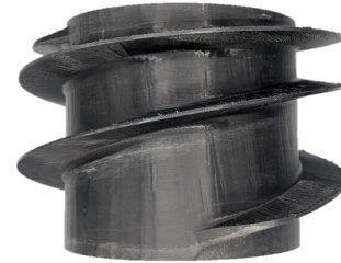
Fig. 8. Example of a screw shell with pitch being changed across the length
