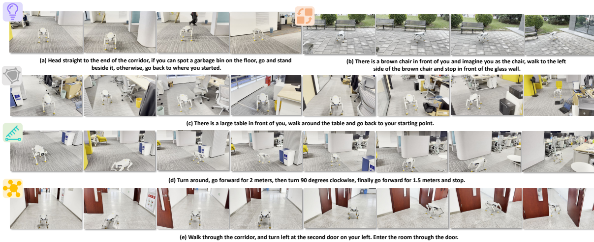
Fig. 6: Qualitative results from the real-world deployment of SNav. The evaluated instructions cover five categories proposed in NavSpace. The test environment includes the office, the campus building, and the outdoor area.
