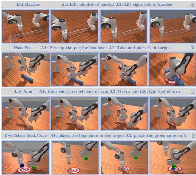
Fig. 6. Dual-arm manipulation tasks. From left to right: Lift Barrier, Pass Peg, Lift Arm, and Two Robots Stack Cube. Each task requires precise coordination between two agents with distinct roles specified through language instructions.
