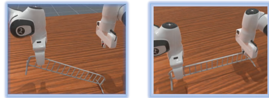
Fig. 8. Left: Shallow grasp causes slipping. Right: Tactile feedback enables more refine, stable grasping.
