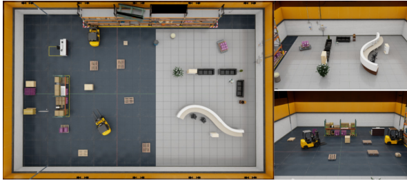
Fig. 4: Residual RL training environment. Multiple instances are tiled and run in parallel to accelerate data collection and model updates.
