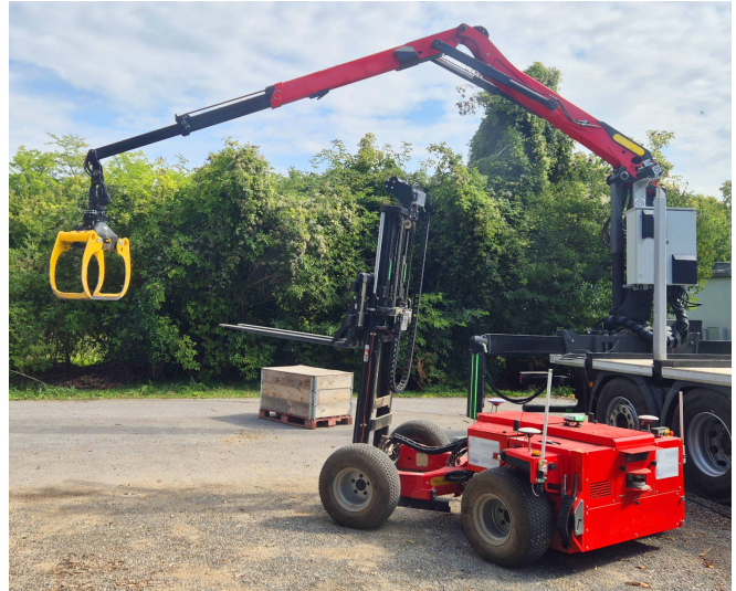
Fig. 2: Image of the autonomous forklift operating in an outdoor environment, where our parametric object detection method is tested and deployed. The main detection targets such as the gripper, loading platform and pallets are visible to provide understanding of the perception task and context.
