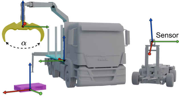
(a) CAD models of the truck-mounted loading crane, forklift, and pallets. Supervision targets: gripper, loading platform, and pallets. Target reference coordinate frames are visualized as well as gripper opening value \alpha . The simulated LiDAR sensor is mounted on the forklift mast, matching the real-world configuration.
