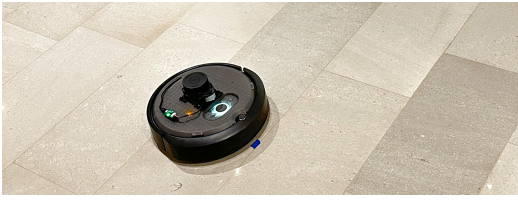
Fig. 4. An image of our iRobot Create 3 in a corridor of map f14 . The RPLIDAR A1 is mounted on top of the robot.
