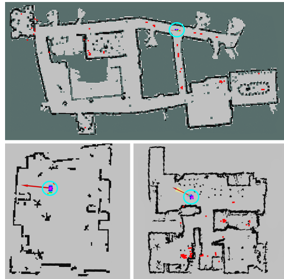
Fig. 1. A demonstration of our algorithm in different real-world scenarios. All images are screenshots from RViz. In all scenarios, the robot uses merely k = 16 distance measurements and its odometry to consistently find its location. All colorful squares are pose candidates returned by our method, where their color ranges from red (least likely) to magenta (most likely). Cyan marks the ground truth location. Top : A large-scale floor plan (f14). Bottom left : A map of our laboratory (lab446). Bottom right : A floor plan of an apartment (apt).
