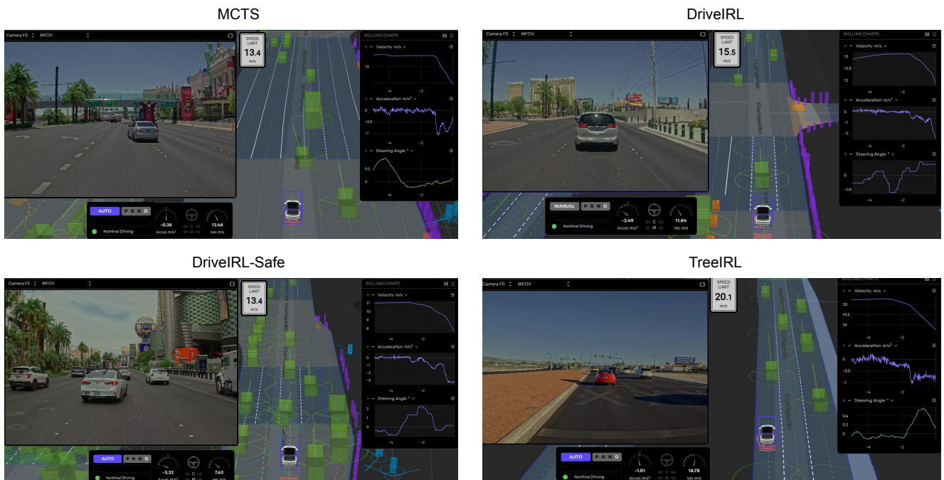
Fig. 6. Cut-in examples from real-world driving. Inset, recent history of AV kinematics. For DriveIRL, t = 0 corresponds to a safety-related takeover (cut-in failure).
