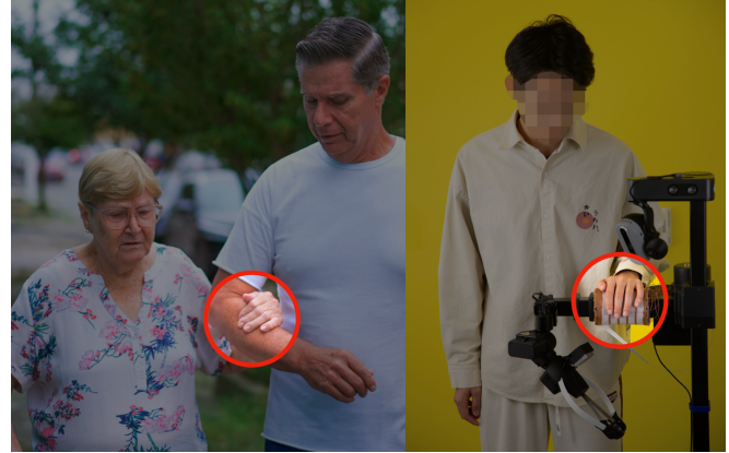
Fig. 1. Intuition of our work: Mobility-impaired people convey their moving intents by applying specific grasping force patterns on the arm of caregiver. We adapt this intuitive and natural way of interaction to the robot assistive navigation by putting a tactile skin on the arm of a Stretch robot.
