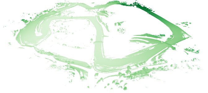
Fig. 4. Dense LiDAR map of the Laguna Seca Raceway from running offline FGO based SLAM framework with color coded by altitude.
