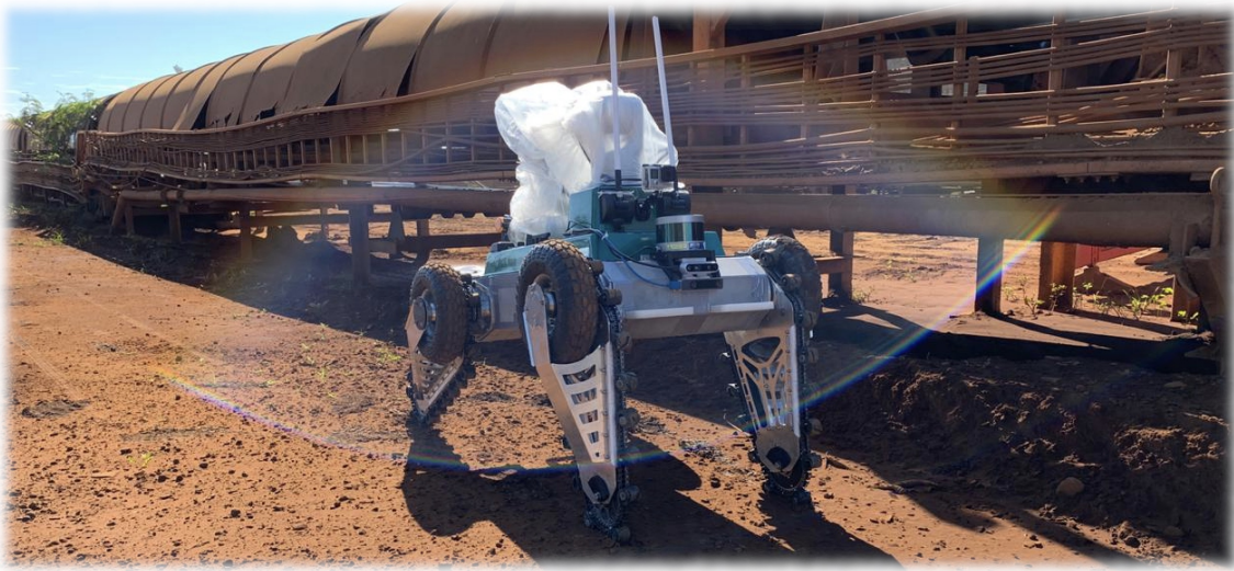
Fig. 1: Hybrid AATV named ROSI developed for belt conveyor inspection. The main locomotion system is wheeled, while tracked flippers are used to overcome obstacles.
