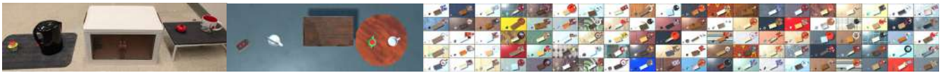
Fig. 6: An emergency stop button, a black kettle, a white container, a small table, a desk bell, a mug. Diverse CLIP+Objaverse [6], [23] reconstructions, generated without human supervision from a ConceptGraph [1] collected using a LoCoBot and an Intel Realsense. The floor colourings were obtained at random from AI2Thor’s [22] large selection of floors.
