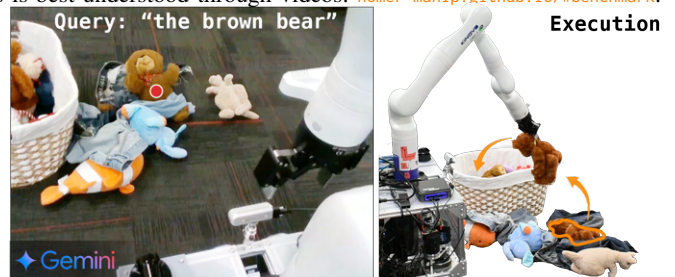
Fig. 6: Real-World Generalization: Left: Given a specified target stuffed animal (“brown bear”), and an image from the base-mounted camera, Gemini identifies an appropriate 2d keypoint (●). Right: Conditioned on this deprojected salient point, HOMER-COND successfully picks up the selected animal and places it in the basket. This illustrates HOMER’s ability to leverage off-the-shelf VLMs for open-set, language-conditioned manipulation.
