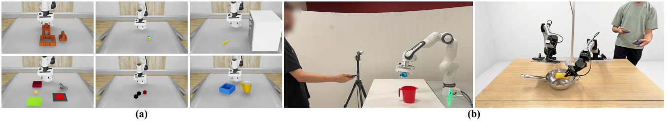
Fig. 5: (a) Visualization of Isaac Lab tasks in the pilot dataset. Arrangement of tasks left-to-right, top-to-bottom: Assembly, Lift, Cleanup, Kitchen, Stack, Pour. (b) COBALT can be used to control physical (single-arm and bimanual) robots. A real-world recreation of the pour task and a corn cooking task are shown.
