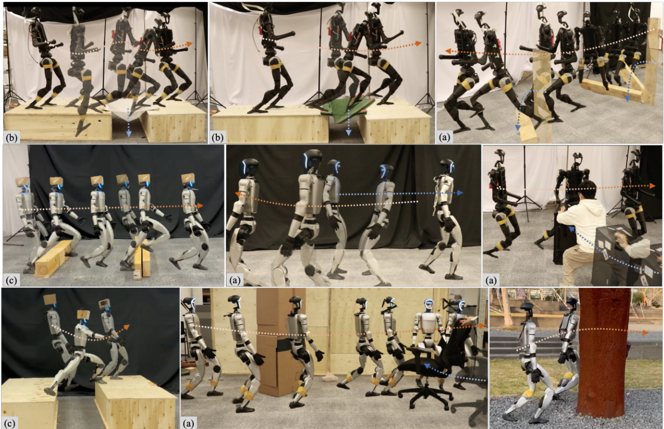
Fig. 1: Overview. VB-Com enables humanoid robots (move direction in orange arrow) to traverse dynamic disturbances (move direction in blue arrow), including (a) suddenly appearing obstacles/hurdles, (b) deformable gaps, and (c) sensor occlusions. We demonstrate the effectiveness of VB-Com on various humanoid robots of Unitree G1 and H1.
