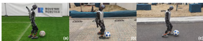
Fig. 6: Dribbling on diverse rough terrains. (a) Artificial Grass, (b) Potholed Ground, (c) Asphalt Pavement.
