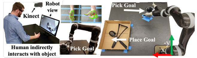
Fig. 6: The studies conducted hands-free teleoperation, where operators could freely move around and an overhead camera collected hand information. We requested recorded operator motion and known goal locations for each scenario. Scenario 1 had a single grasping point (central robot photo), while scenario 2 contained two goals including a pick and place goal (right robot photo).
