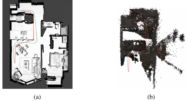
Fig. 5: Results from the Swormville scene (Gibson dataset). (a) Top-down map showing the ground-truth shortest path (—) and the executed risk-averse trajectory (—). (b) 3-D Gaussian-splat reconstruction of the scene; only the forward-looking masked region relevant to the task was used for learning, illustrating the sparse, task-focused sensing.
