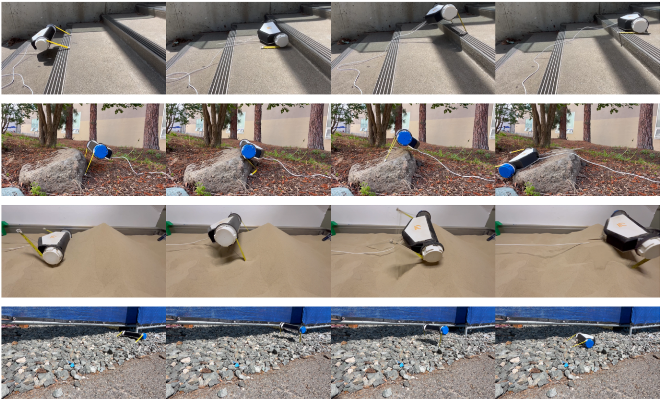
Fig. 9. The stowable tape spring truss rover traversing obstacles such as stairs, rocks, sandy mounds, and rubble, which would otherwise it was not able to traverse in the wheeled setting.
