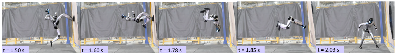
Fig. 6: Hardware results showing a high-dynamic wall-flip motion. The robot reaches a maximum linear velocity of 3.5 m/s and a peak angular velocity of 15 rad/s.
