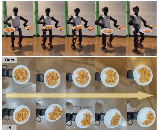
Fig. 4: Plate holding task. With our method, the robot can stably hold the plate without spilling the snacks, whereas the IK-based method causes noticeable end-effector oscillations, leading to significant spillage.
