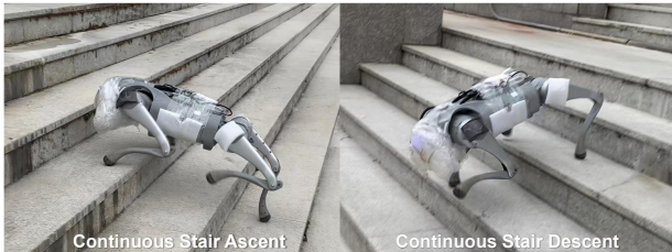
Fig. 5: Real-world experiments: continuously ascending and descending multiple high steps. For more scenarios, gait details, and the complete experimental process, please see the supplementary video.
