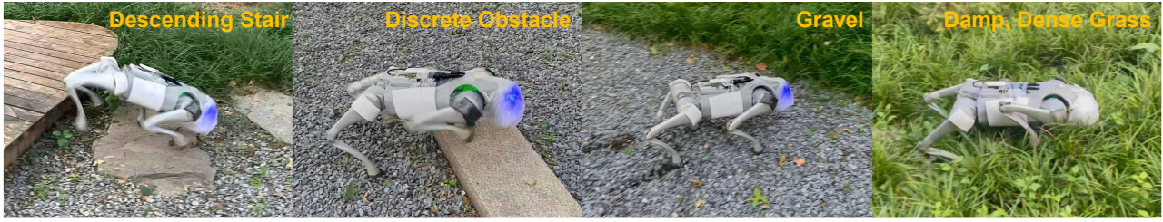
Fig. 2: The robot traversing a continuous segment of challenging mixed terrains, including descending stairs, discrete obstacles, gravel, and a damp, dense grassy area.
