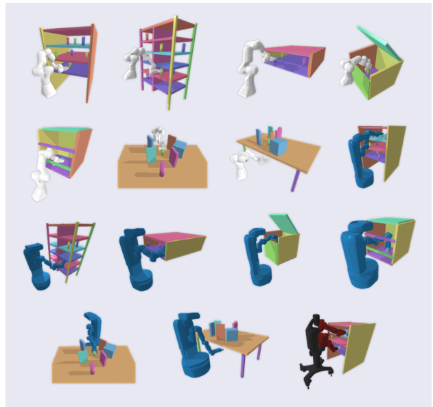
Fig. 2: The MotionBenchMaker scenes provide diverse manipulation problems for 7, 8, and 14 DoF robots. The problems include counter top manipulation, accessing shelves, and constrained reaching. Panda and Fetch have 7 scenes with 100 problems each, while Baxter has 3 scenes with 500 problems each.
