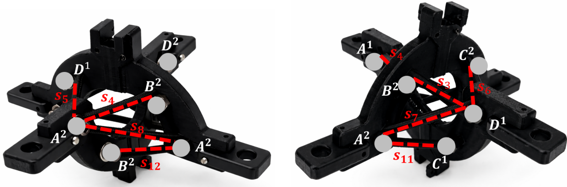
Fig. 3. (left) Front and (right) Back view of the tensegrity sub-vertebra with compressive members and tensile connection strings.
