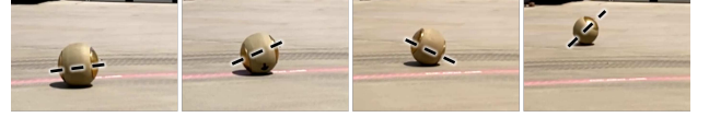
Fig. 7. Screenshots of the shell experiencing a nutation instability, the hubcaps start parallel to the viewer, then start relaxing toward perpendicular while maintaining a steady path away
