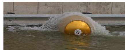
Fig. 12. Robot rolling in water with \omega_2 around 18 rad/s
