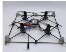
(a) Lifting robot: a customized platform built on Crazyflie Bolt, designed to grasp the cable endpoints and maintain global tension.
