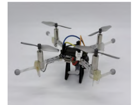
(b) Support robot: Crazyflie 2.1 nano quadrotor, used as an intermediate robot to regulate cable spans.
