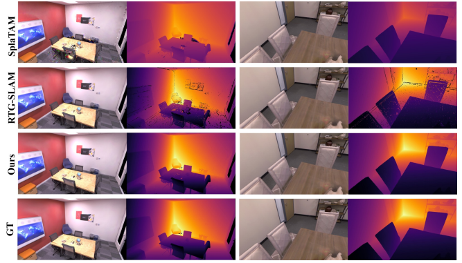
Fig. 4: Qualitative results of color and depth rendering in S 3 LAM compared to representative 3DGS-based methods. Our method exhibits fewer artifacts and clearer borders in the rendered color and depth.
