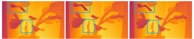
Fig. 6: Qualitative ablation results: Depth reconstruction without the adaptive strategy using mean depth ( Left ), with our proposed distortion-based adaptive strategy ( middle ), and the ground-truth depth ( right ).
