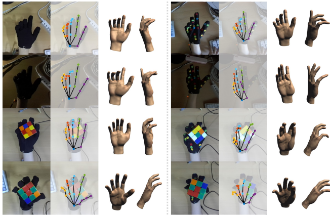
Fig. 8. Tracking results of our framework (left) and VIST (right). The top two figures show hand pose estimations before (1st row) and 5 minutes after (2nd row) the illumination change. The bottom two figures illustrate estimations with object interaction.
