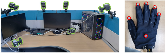
Fig. 6. Motion capture setup for quantitative evaluation. We use six calibrated IR cameras (left figure; highlighted in green) and six reflective markers attached to the glove (right figure; marked in red).
